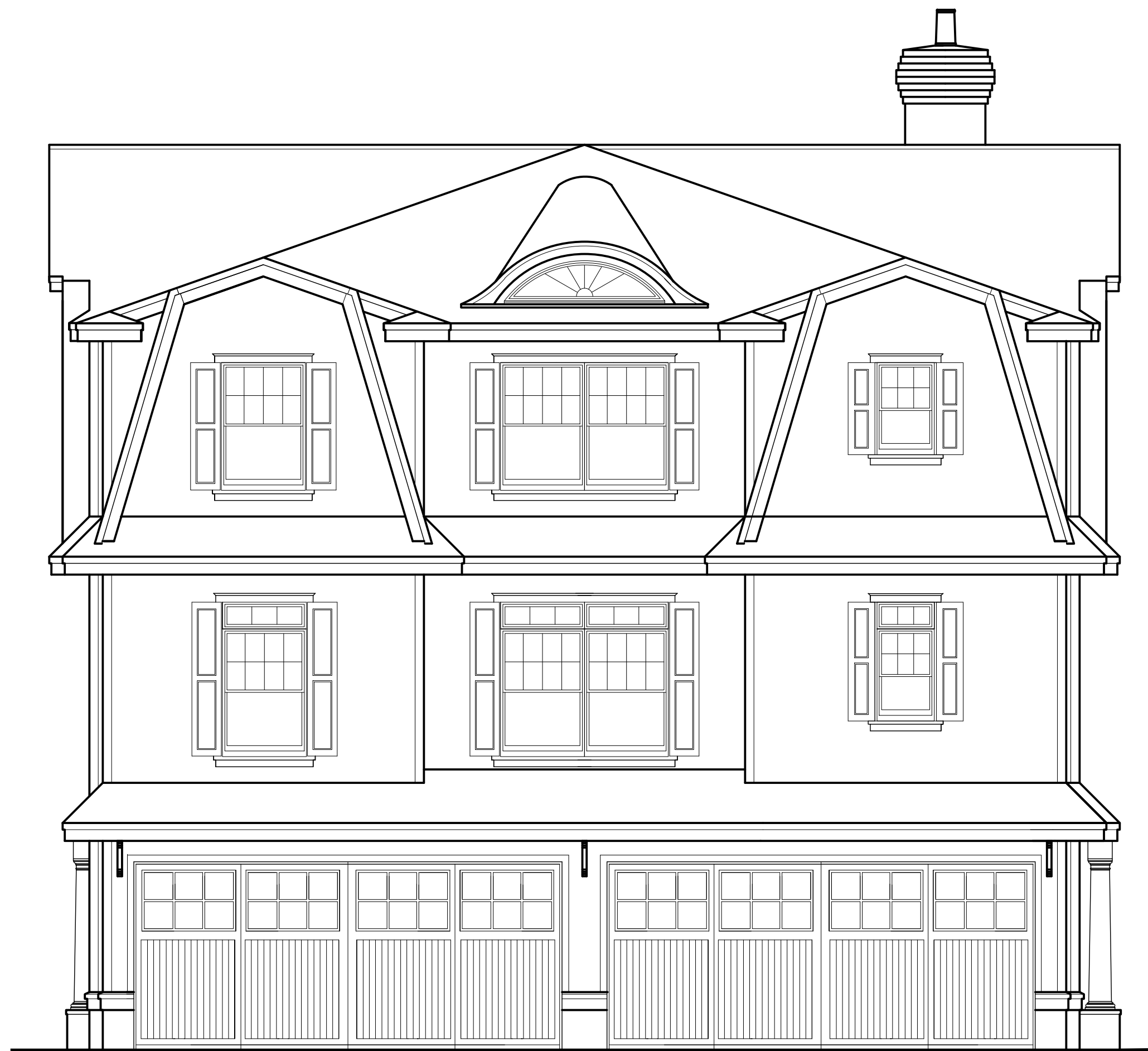
3 FRONT ELEVATION DD SCALE: 1/4" = 1'-0"
